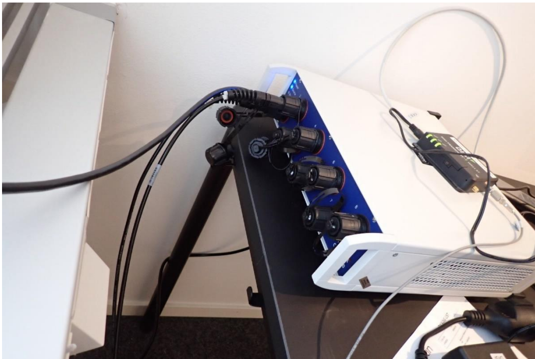
Figur 14: Interrogator. 50 m stand-off cable kopplas in här
